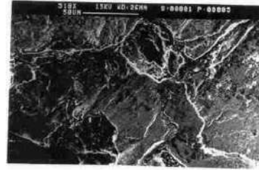
Fig. 4. Fractograph of the failed crankshaft shows that failure initiated from transition region from grooves that contained surface discontinuities (a-e) and progresses in the web region.
