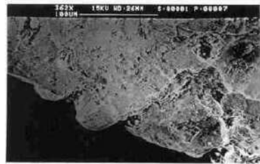
Fig. 4. Fractograph of the failed crankshaft shows that failure initiated from transition region from grooves that contained surface discontinuities (a-c) and progresses in the web region.
