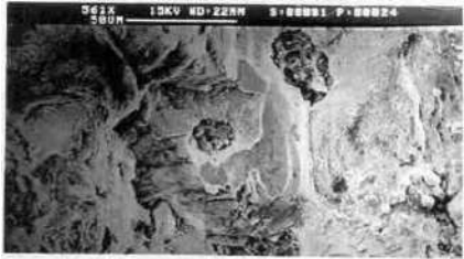
Fig. 4. Fractograph of failed crankshaft shows a number of secondary cracks, porosities and nodule separation at the matrix interface (h & i).
