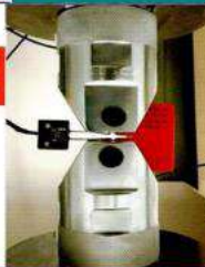
Fracture Toughness (CTOD) of 3D Printed PLA Sample
