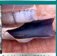
Typical burst failures CNG Cylinder.
